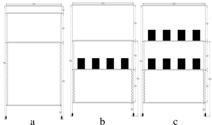
Figure 2: A graphical presentation of designed cart. a: empty, b: one shelf loaded, c: two shelves loaded
